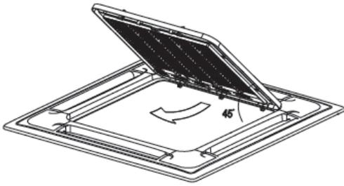
**(2) Remove the installation covers at the four corners.**
